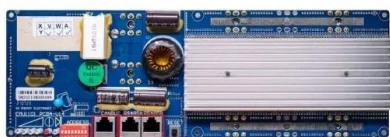
RS485 Interface Communication between battery and inverter Read rate: 9600bps RS485 Interface Communication between parallel packs or EMS and PC Read rate: 9600bps
